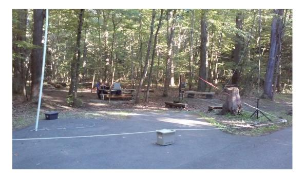
The photo from the first test in the series (Courtesy of Terry Carnahan-KB3JOD) shows the typical setup for the NVIS (white pole) and the 2m antenna at site alpha. Doug is sitting at the table and the radios are provided by Terry C.
